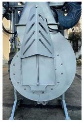
The new centrifugal fan in steel sheet  $\emptyset$  570 mm ensures first-rate performance, thanks also to the oversized 825x250x500 mm casing and  $\emptyset$  200 mm ducts. This allows the POWER MULTIROW to move an air volume that can reach 22,000 m<sup>3</sup> / h at extremely high speeds.
